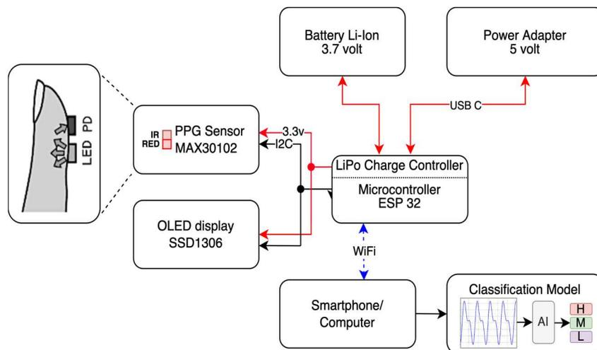
Fig. 1 A non-invasive prototype [14] was used to record PPG signals.
