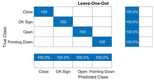
Fig. 15 Confusion matrix for front side radar
