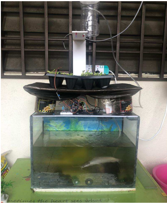
Fig. 5 Prototype of the smart automation aquaponic monitoring system
