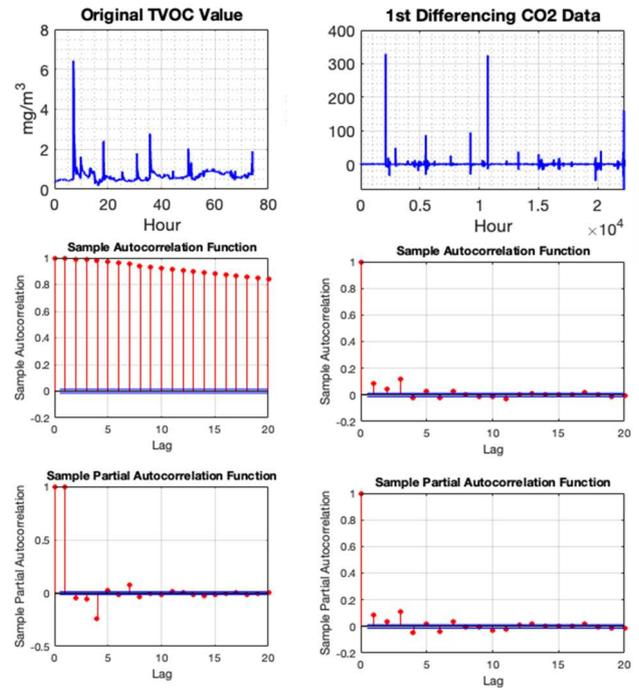
Fig. 8 Left: TVOC uses order 0 or data origin to determine AR and MA. The spike on PACF is at lag 1 and ACF is at lag 1, thus AR=1 and MA=1. Right: while for CO<sub>2</sub>, a differencing process must be carried out to obtain ACF and PACF. Spike on PACF is at lag 3 and ACF is at lag 3, thus AR=3 and MA=3
