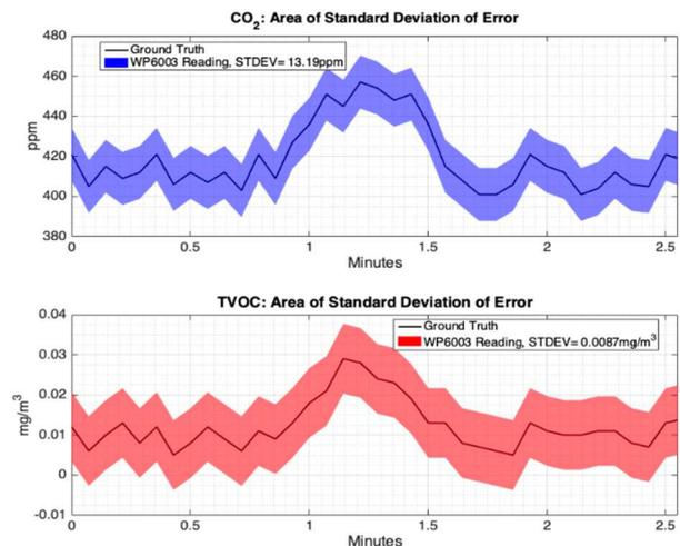
Fig. 6 Error in readings between the sensor devices used (WP 6003) compared to the commercial sensor IAQI JD032 series
