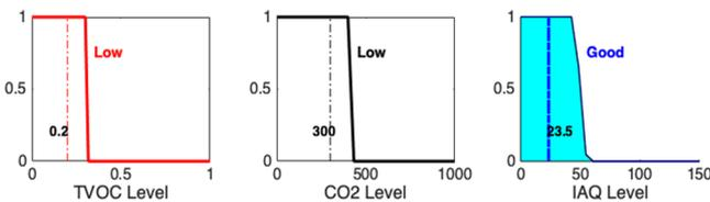
Fig. 4 Input membership function and the output of defuzzification
