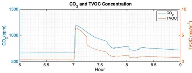
Fig. 7 Two condition applies: normal indoor air quality (hour 6 to 7), adding aerosol changes the normal condition to high polluted indoor air (hour 7 to 8).
