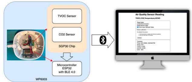
Fig. 5 Architecture and desktop application to read data from sensors
