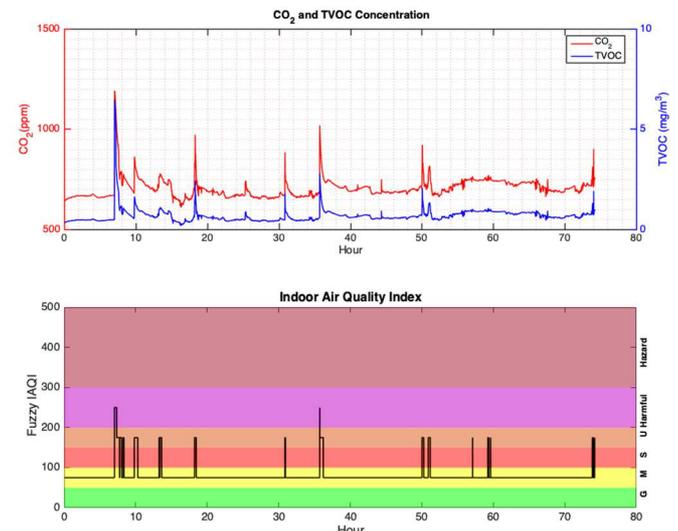
Fig. 10 TVOC and CO<sub>2</sub> time series dataset obtained by the sensor for about 74 hours. Below: FIAQI outputs.
