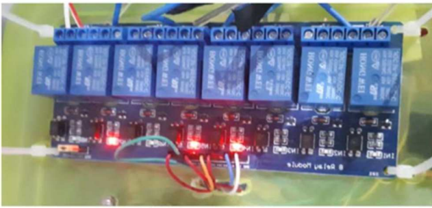
Fig. 8. The actuator response: nutrient A pump on, nutrient B pump on, and water cooler on.
