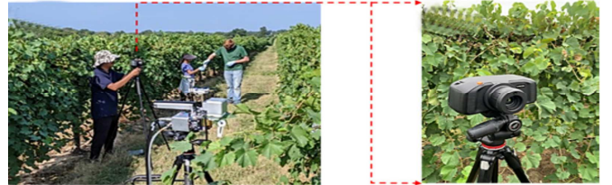
Fig. 1 SPECIM IQ sensor mounted on a tripod (left). (right) A close-up of the SPECIM IQ sensor [10].
