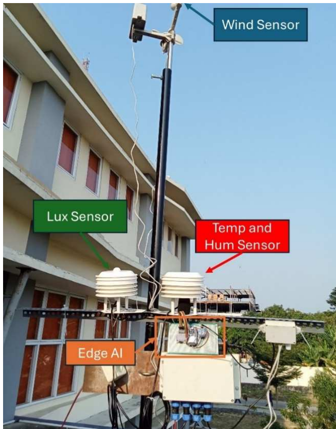
Fig. 7 Overview Rainfall Prediction Application with weather sensor and edge AI for this implementation
