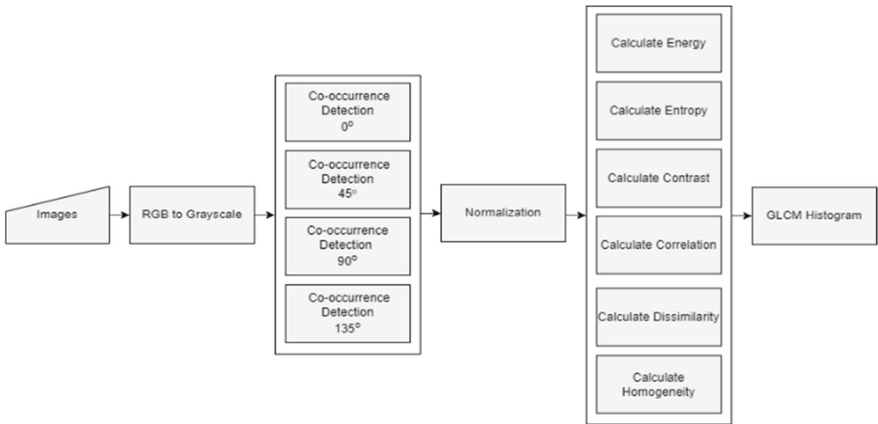
Fig. 9 Illustration of GLCM features extraction.
