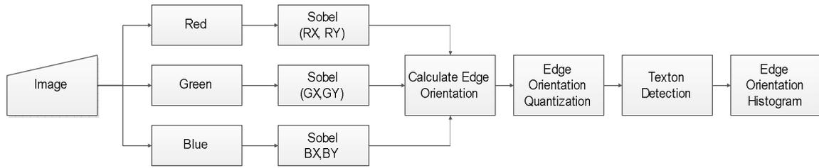
Fig. 4 Illustration of edge features extraction
