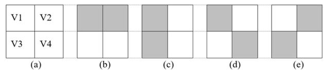
Fig. 2 Four types of texton on MTH. (a) 2x2 Grids; (b) T1; (c) T2; (d) T3; (e) T4
