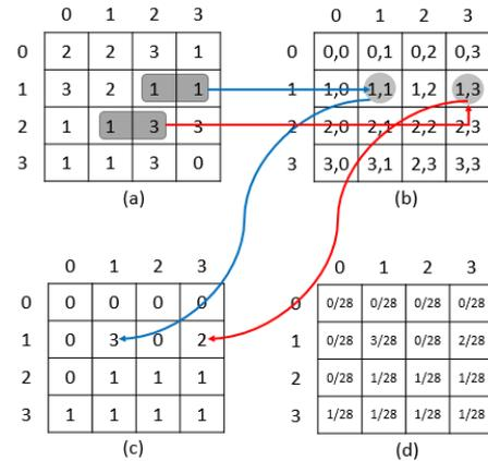
Fig. 1 Illustration of GLCM feature extraction (a) grayscale image; (b) definition of reference matrix; (c) reference matrix; (d) matrix normalization
