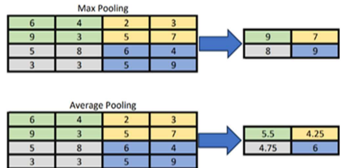
Fig. 3 Max Pooling and Average Pooling
