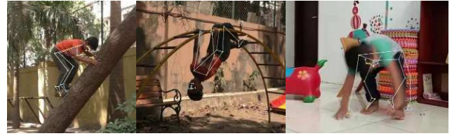
Fig. 5 Skeleton keypoints were overlaid on video clips processed by MediaPipe and then quantized.
