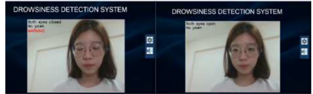
Fig. 16 Sample screenshot of the drowsiness detection system graphical user interface
