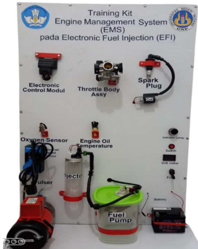
Fig.1 Electronic Fuel Injection (EFI) fuel system simulator on a motorbike
