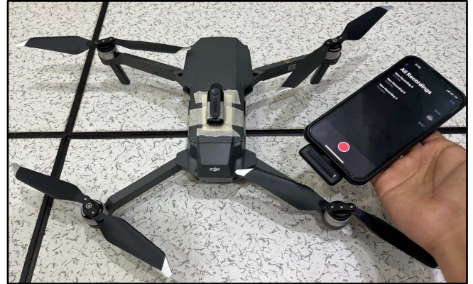
Fig. 3 Setup of drone and microphone
