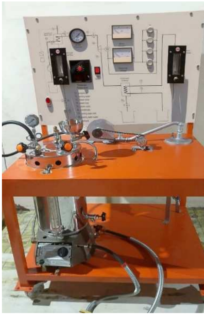
Fig. 3 Steam Power Plant Trainer
