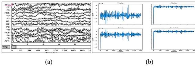
Fig. 3 EEG signals: (a) before being given a high-pass filter and (b) after being given a high-pass filter
