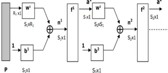
Fig. 2 Diagram of Multi-layer perceptron
