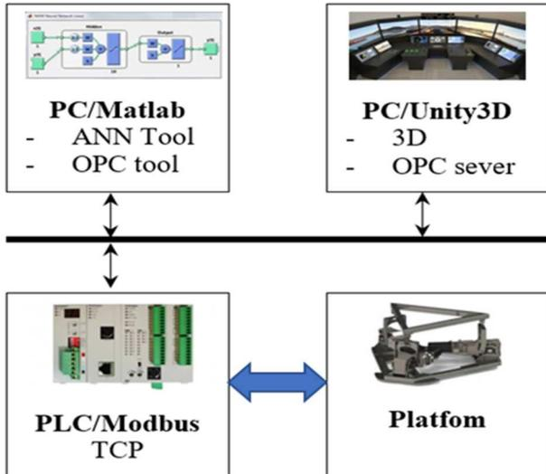
Fig. 3 Structure diagram of Cockpit cabin deck with integrated ANN/MLP module
