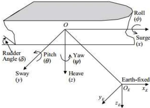
Fig. 1 Ships' kinematic parameters and motion components in the horizontal plane
