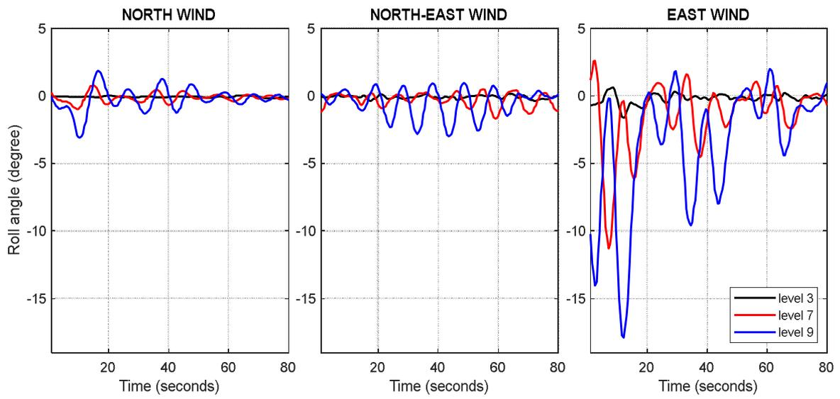
Fig. 7 Record of the roll angle of the platform
