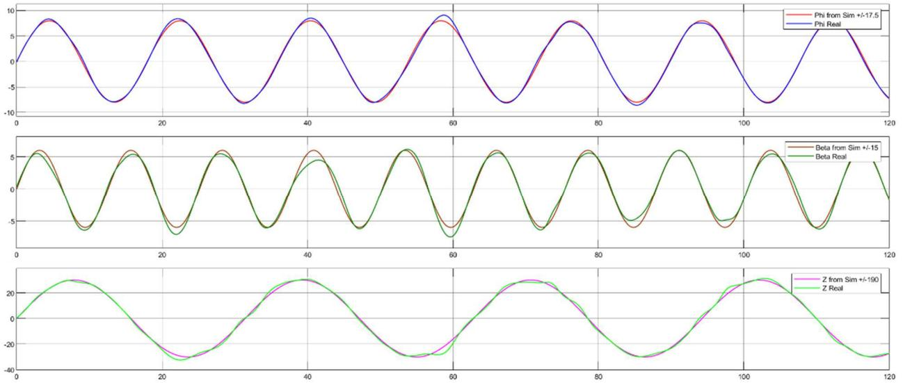
Fig. 12 In the presence of a neural network, the output signal simulation's  $\phi$  (roll),  $\theta$  (pitch), and z (heave)
