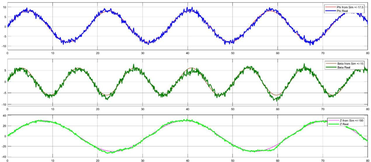
Fig. 14 The output signal simulation's  $\phi$  (roll),  $\theta$  (pitch), and z (heave) in detail
