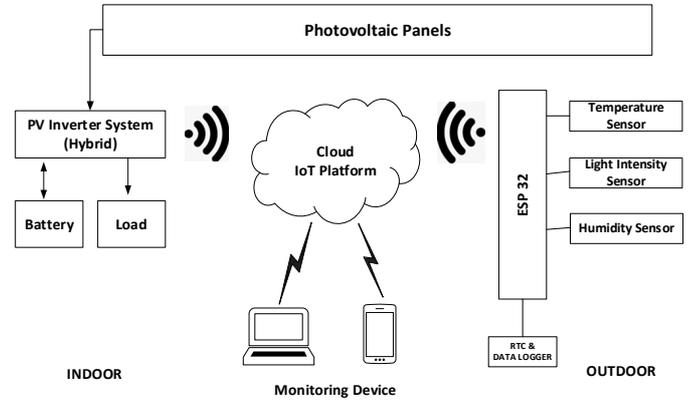
Fig. 1 The system architecture of data collection
