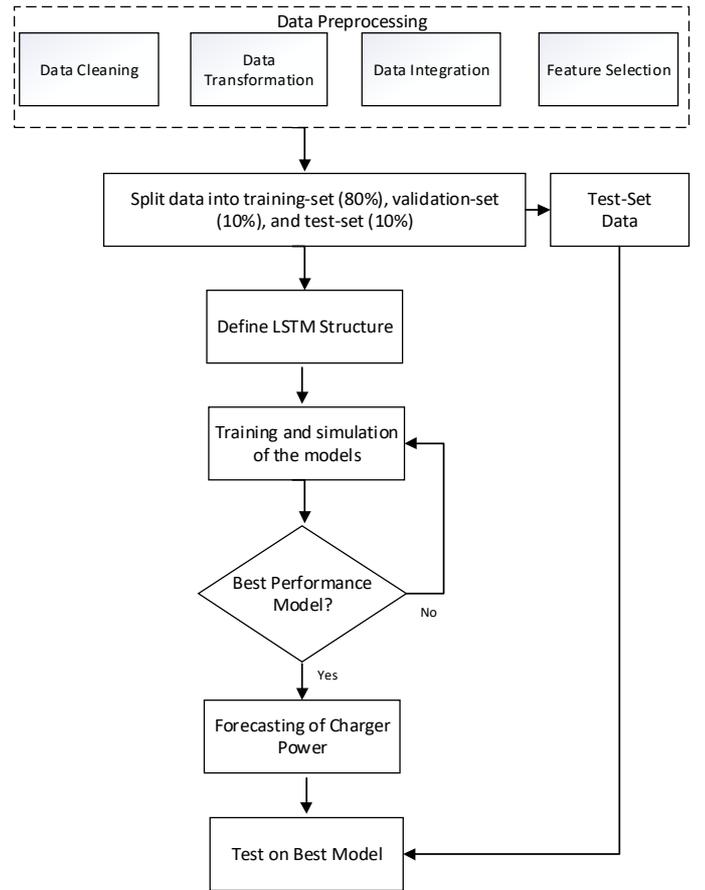
Fig. 3 Forecasting flowchart Charging in PV system.
