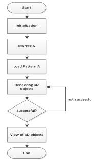
Fig. 2 Flow Chart from Marker Based AR
