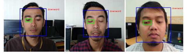
Fig. 9 Several results of downward detection using Backpropagation Neural Network
