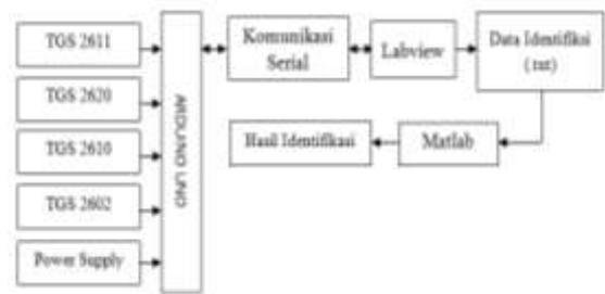
Fig 2. Block Diagram Process
