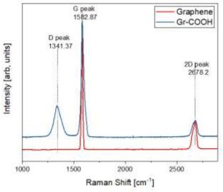
Fig.4. Raman spectra of Graphene (red line), Gr-COOH (blue line)
