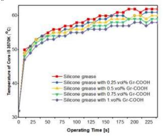
**Fig.7.** The measured temperature of the microprocessor as a function of the operation time in the case of using thermal grease
