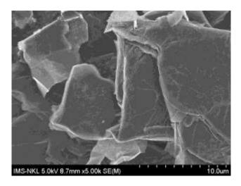
Fig.3. FESEM image of graphene nanoplatelets
