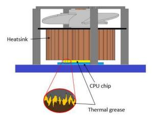
Fig.2. Scheme of the cooling system using thermal grease containing Gr-COOH
