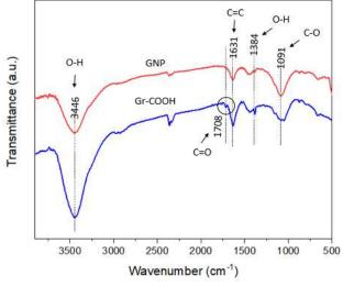
Fig.5. FTIR transmission spectra of pristine GNPs, Gr-COOH.
