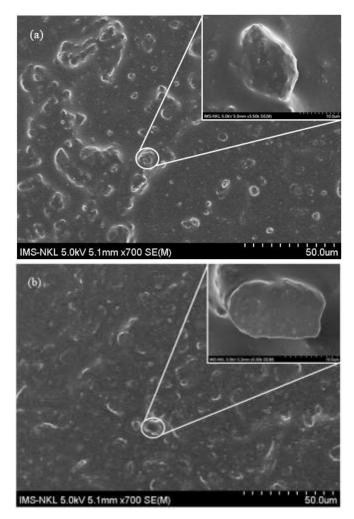
**Fig.6**. FESEM image of silicone thermal grease (a) and silicone thermal grease containing Gr-COOH (b)
