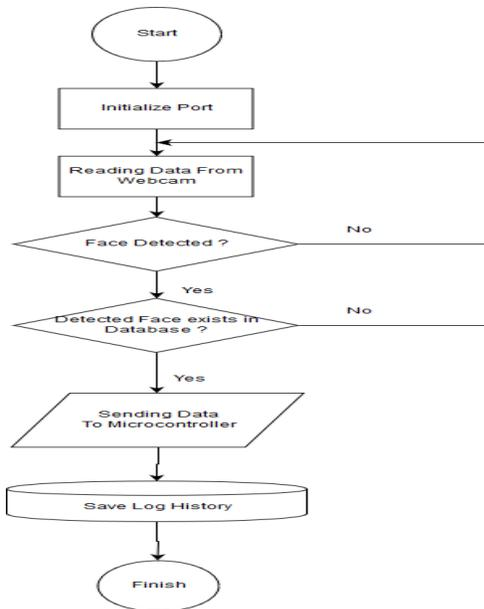
Fig 5. Flowchart Arduino Application
